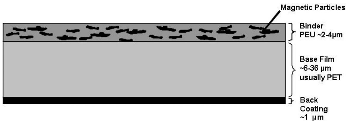
Figure 1. Audio magnetic tape cross section.
